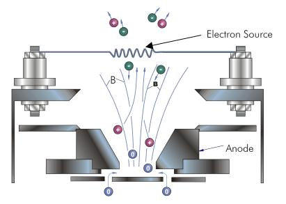
Gridless End-Hall ion sources provide an accelerating potential using both magnetic and electrical fields. The gridless design enables the source to generate high currents (up to 5A), low energy beam for wide area coverage.
