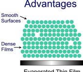
Evaporated Thin Film with Ion Beam Assist
