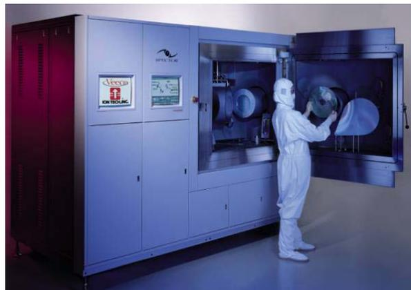
The SPECTOR<sup>®</sup> dual ion beam deposition system, utilizes the best RF ion source technology on the market, providing unmatched deposition rate, uniformity and film quality control. SPECTOR was recently combined with new process technology to
